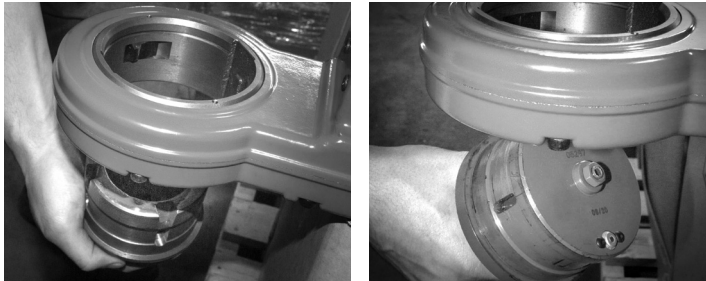
Both the TMPDA and VOKUCLUTCH install in the same orientation.
