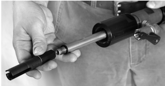
Attach coupling nut to shell cutter.
