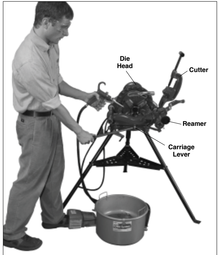
Figure 9 - Threading Pipe with R811 Die Head
